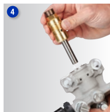
Install new cartridge and replace pump
